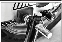
Align the paddles directly underneath the bikes rear swingarm, push down, and motorcycle will lift. (Spools are not required)
