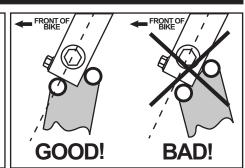
Confirm that the width of the fork attachments are at the correct distance for your bike. Align the lower pad with the forks centerline (see example above)
